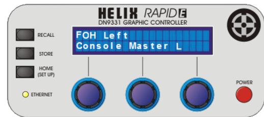
In the Graphic EQ Channel Display, none of the encoders is active.
