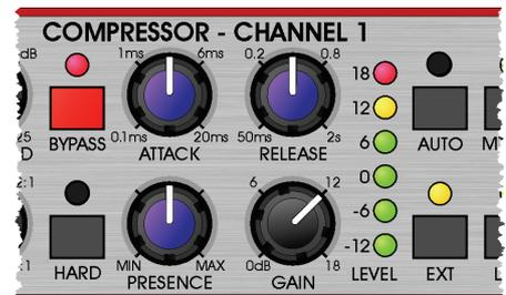
The compressor normally sounds best on applications that require slower attack time settings. If faster attacks are needed it is normally best to switch on the hard knee.
