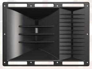
is a proprietary coupling device that introduces driver output to the horn throat across a very short path (3 inches for the mid-high section and 1.5 inches for the very-high section), effectively controlling the output but with dramatically reduced distortion in comparison to other techniques.
