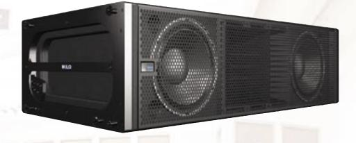
MILO's rigid cabinet is constructed from multi-ply hardwood and steel braced for long-term durability in touring applications. Sturdy rigging frames ensure ease of flying or stacking, and also keep stresses outside the enclosure. Integral power amplification and control electronics are optimally matched to transducers to maximize the power-to-size ratio.
