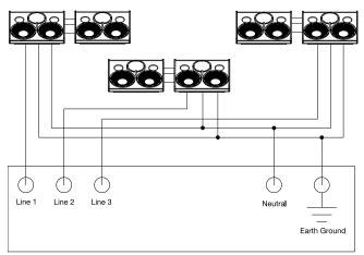
Figure 2.1. A sample AC power distribution block diagram
