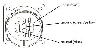
For complete wiring conventions and pin-outs for AC, audio, and RMS connections, please refer to the Meyer Sound document VEAM Cable Wiring Reference (PN 06.033.113.01).
