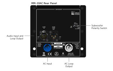
The audio input shall be electronically balanced with a 10-kOhm impedance and accept a nominal -2.0 dBV (0.8 V rms, 1.1 V peak) input signal. Connectors shall be XLR female for input and XLR male for loop output. De blocking and RF filtering shall be provided, and CMRR shall be greater than 50 dB and typically 80 dB (50 Hz to 500 Hz).
