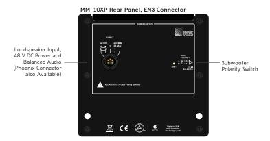
The loudspeaker shall be equipped with either a Phoenix 5-pin male or EN3 5-pin male connector (three pins for balanced audio and two pins for DC power). The audio input shall be electronically balanced with a 10-kOhm impedance and accept a nominal -2.0 dBV (0.8 V rms, 1.1 V peak) input signal. DC blocking and RF filtering shall be provided, and CMRR shall be greater than 50 dB and typically 80 dB (50 Hz to 500 Hz).
