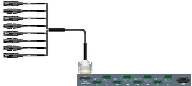
3. Connect audio sources (from a mixer or processor) to the other end of the audio cable or snake.
