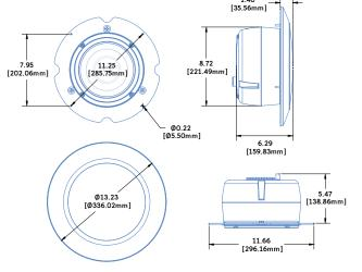
The Stella-8C ceiling mount installation loudspeaker is a self-powered loudspeaker engineered primarily for use in Meyer Sound's Constellation electroacoustic architecture. Housed in an aluminum die cast enclosure with a heatsink on the back, the Stella-8C can be flush-mounted in ceilings and walls with standard backboxes for 8-inch drivers (with a minimum depth of 6.5 inches).
