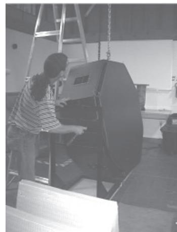
With the speaker suspended the yoke can be easily removed or installed on the speaker.
