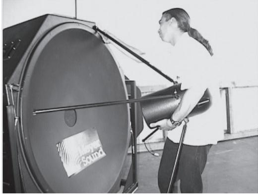
While keeping a firm grip on the pod insert one of the legs into a c-bracket so that the holes in the legs are aligned with the holes in the c-bracket. Then insert a pin through the holes while pressing down on its button head. When the first pin is in position attach the leg opposite to the first one. Repeat this process until all four legs are attached.
