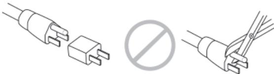
Do not use a ground-lifting adapter or cut the AC cable ground pin.
