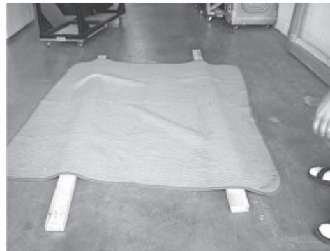
With the protective cover over the dish lie the SB-1 down on the boards so that the rigging points are between the two boards and the amplifier is facing upwards.
