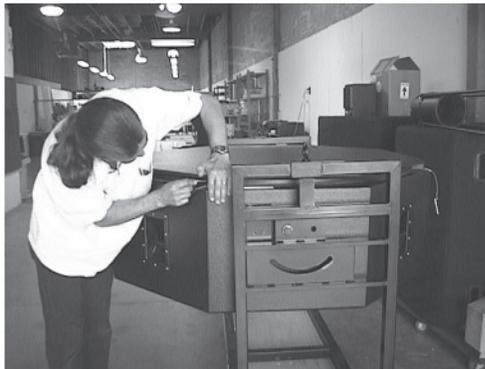
While pressing down on the cover, push the button at the top of the pin in, while pulling the pin out of the C-bracket.
