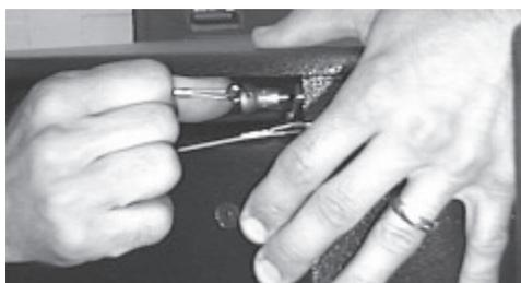
Once each of the pins are removed, the cover can be easily lifted off the SB-1.
