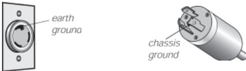
The SB-1 requires a grounded outlet. Always use a grounding adapter when connecting to ungrounded outlets.
