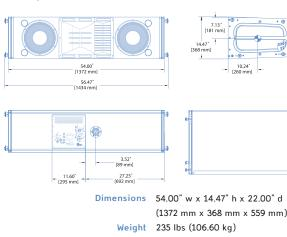
Enclosure Multi-ply hardwood Finish Black textured Protective Grille Powder-coated hex-stamped steel Rigging MRF-MILO rigging frame, custom AlignaLink connectors and quick release pins
