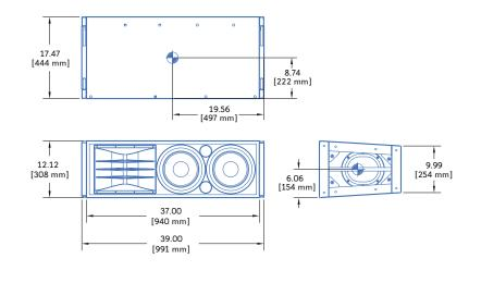
Dimensions39.00" w x 12.12" h x 17.47" d<br/>(991 mm x 308 mm x 444 mm)Weight116 lbs (52.62 kg); shipping: 130 lbs (58.97 kg)EnclosureMulti-ply hardwoodFinishBlack texturedProtective GrillePowder-coated hex stamped steelRiggingPatented QuickFly MRF-2D rigging frame with<br/>integral CamLinks™, rear connecting bars and<br/>captive quick-release pins
