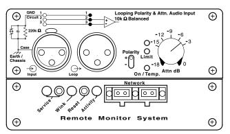
User Panel with RMS option and Polarity and Attenuaing Audio Input Module
