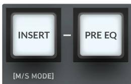
Fusion features a stereo insert point, which provides the ability to introduce other outboard processors such as the SSL G-Series Bus Compressor. The insert point is engaged via the front panel **INSERT** switch and will light bright white when operating in standard stereo mode. The **PRE EQ** switch allows for the insert point to be moved before the **VIOLET EQ** section in the signal path.
