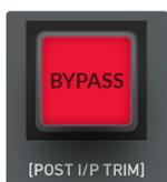
The **BYPASS** switch allows you to bypass all of Fusion's processing blocks. If the **BYPASS** switch is red, then you are in standard **BYPASS** mode. Use this to compare the sound of the mix with/without Fusion in one easy action. It dimly lights white if you are not in bypass.
