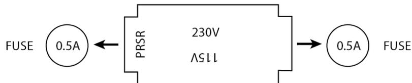
4. Re-orientate the fuse cartridge 180 degrees and place the new 1A fuses in the vacant slots on the cartridge.
