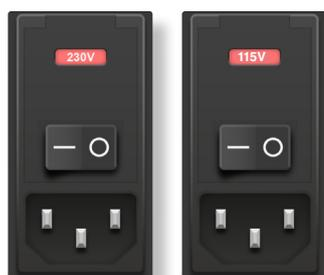
Fusion has a linear power supply and therefore needs to be manually switched to operate with either a 230V or 115V power supply. The AC mains fuse is located on the rear panel next to the AC mains connector. The orientation of the main fuse cartridge will dictate the operational voltage; this can be either 230V or 115V AC power.
