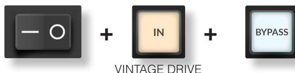
Factory Reset allows reset of any stored settings (Brightness, Relay feedback, **BYPASS** and **INSERT** configurations) to the factory default. Press and hold the combination of switches until all the switches start flashing. After releasing the switches, the unit will automatically reboot and the factory settings will be restored.
