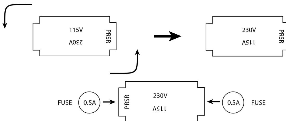
5. Place the cartridge back in the holder so that the 230V value is displayed through the slot in the fastening. Re-seal the fastening, reconnect the IEC power cable, and switch the unit on.
