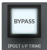
Pressing and holding the **BYPASS** switch for two seconds will cause it to enter **POST INPUT TRIM** bypass mode. You will know because the front panel switch will turn bright white. In this mode, the **INPUT TRIM** pot still affects the sound, even in bypass. This mode is a useful extra feature if you've had to make-up or take off significance amounts of gain using the **INPUT TRIM**.
