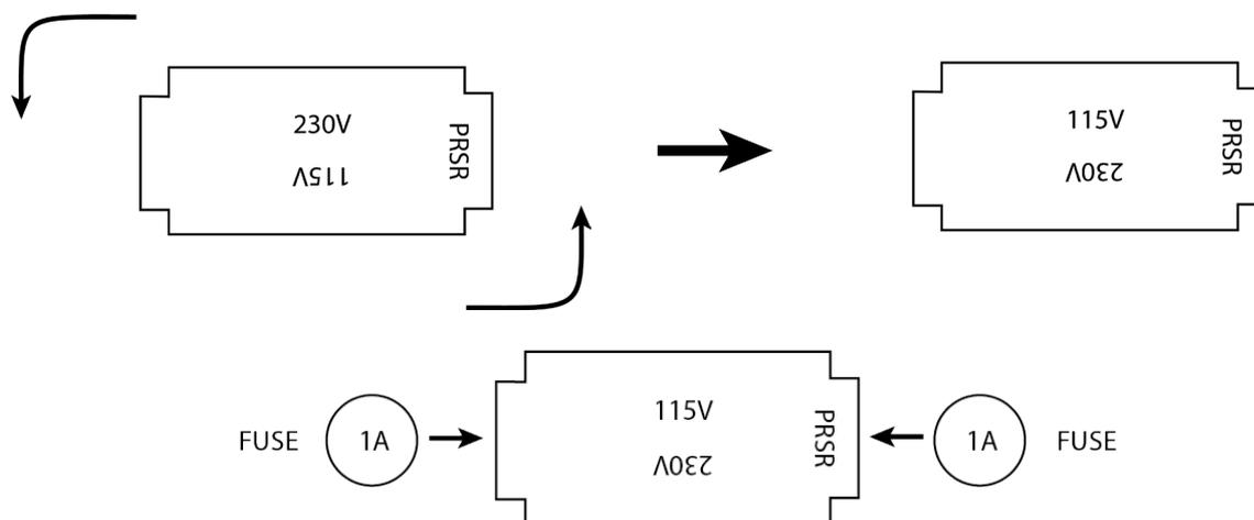
5. Place the cartridge back in the holder so that the 115V value is displayed through the slot in the fastening. Re-seal the fastening, reconnect the IEC power cable, and switch the unit on.
