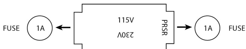
4. Re-orientate the fuse cartridge 180 degrees and place the new 0.5A fuses in the vacant slots on the cartridge.
